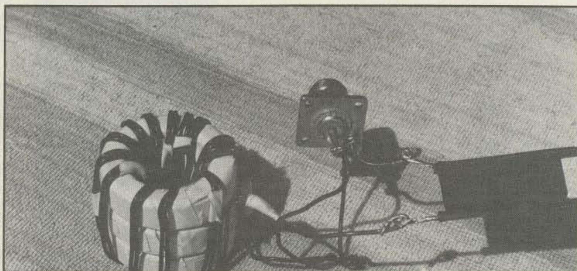
I have deliberately left this "open" type construction to show the bifilar windings and the connections to the coax fitting (SO-239 type) and the other two leads connected to the open-wire line. While electrically this would work well, in actual practice the transformer needs to be mounted in a box or case that is weatherproof.
